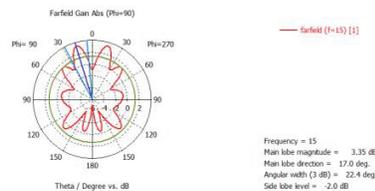
Fig. 12: Gain of 1st iterated fractal patch in stacked structure
