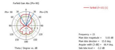
Fig. 8: Gain of stacked square patch antenna
