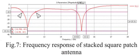
Fig.7: Frequency response of stacked square patch antenna
