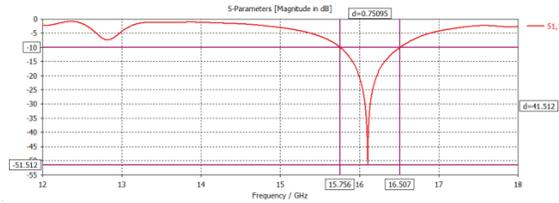
Fig. 9: Frequency response of 1st iterated fractal patch
