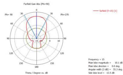
Fig.14: Gain of 2nd iterated of fractal patch
