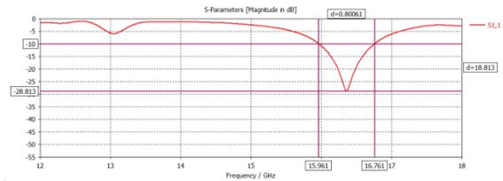
Fig.13: Frequency response of 2nd iterated fractal patch
