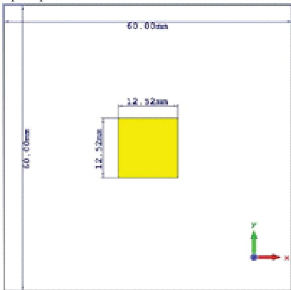
Fig. 1: Square patch antenna
