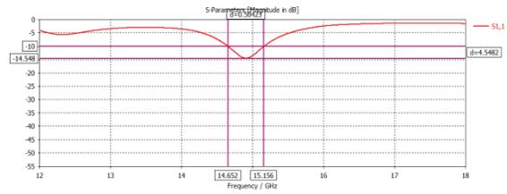
Fig. 5: Frequency response of square patch antenna
